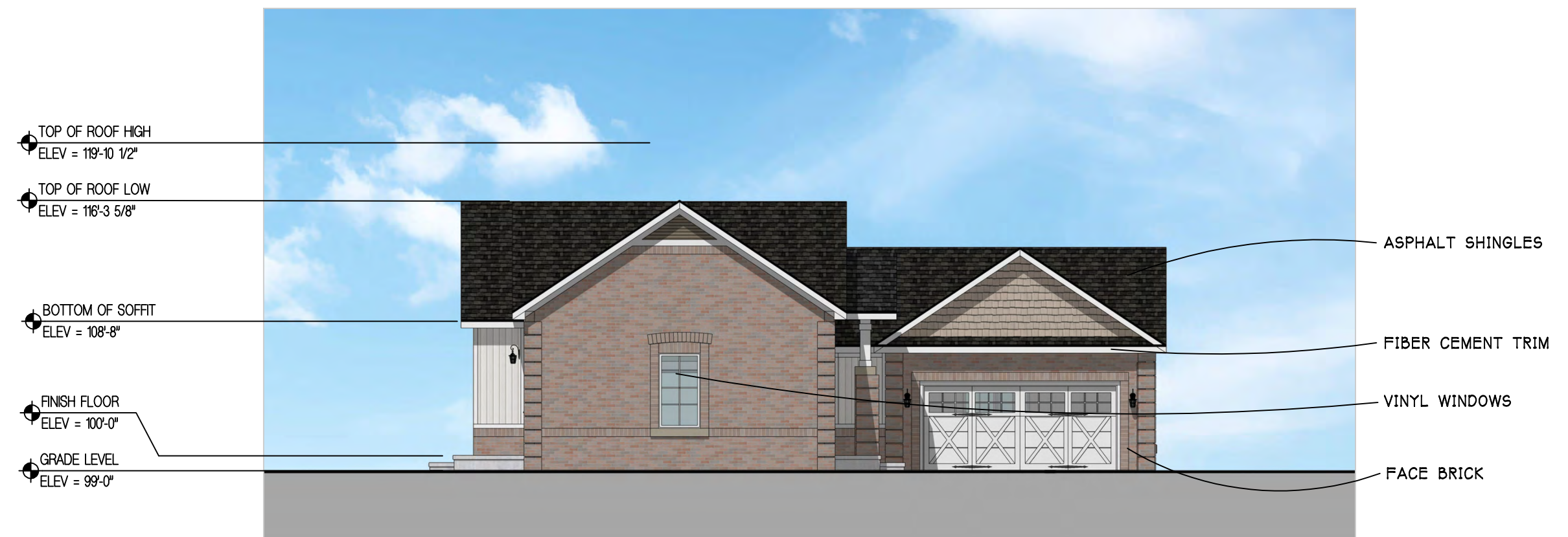
SIDE A ELEVATION UNIT B SCALE - 1/8" = 1'-0" SASHA1202
