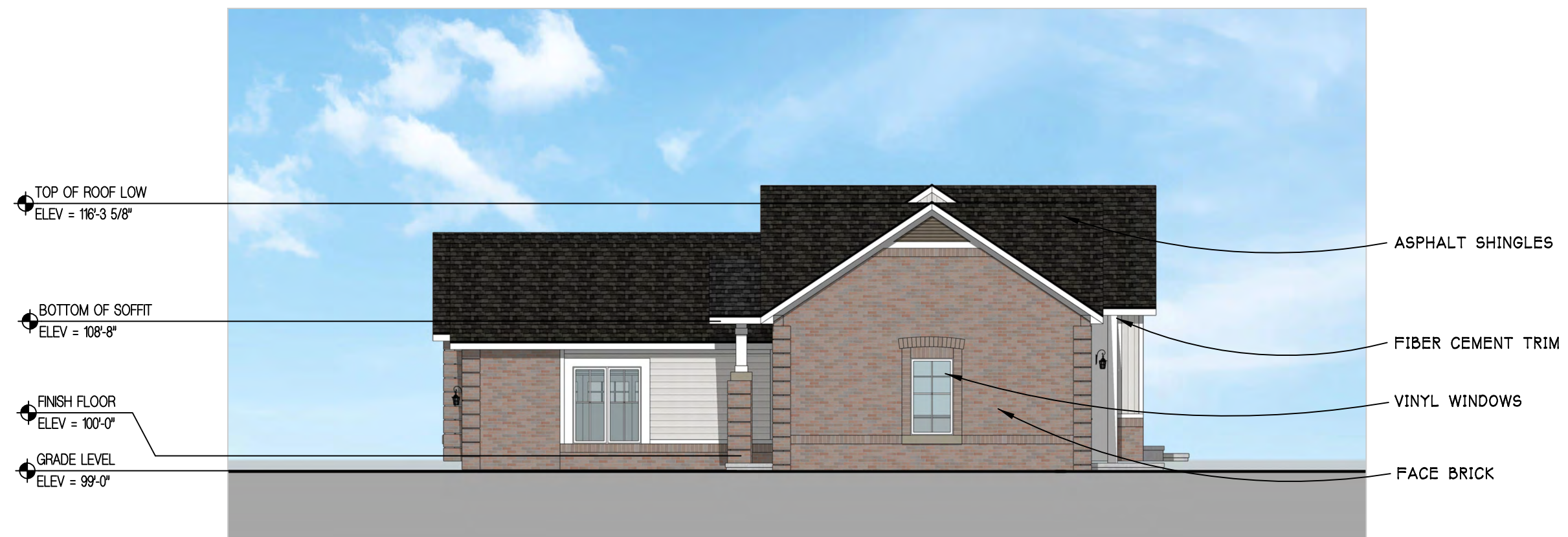
SIDE B ELEVATION UNIT B SCALE - 1/8" = 1'-0" SASHA1202
