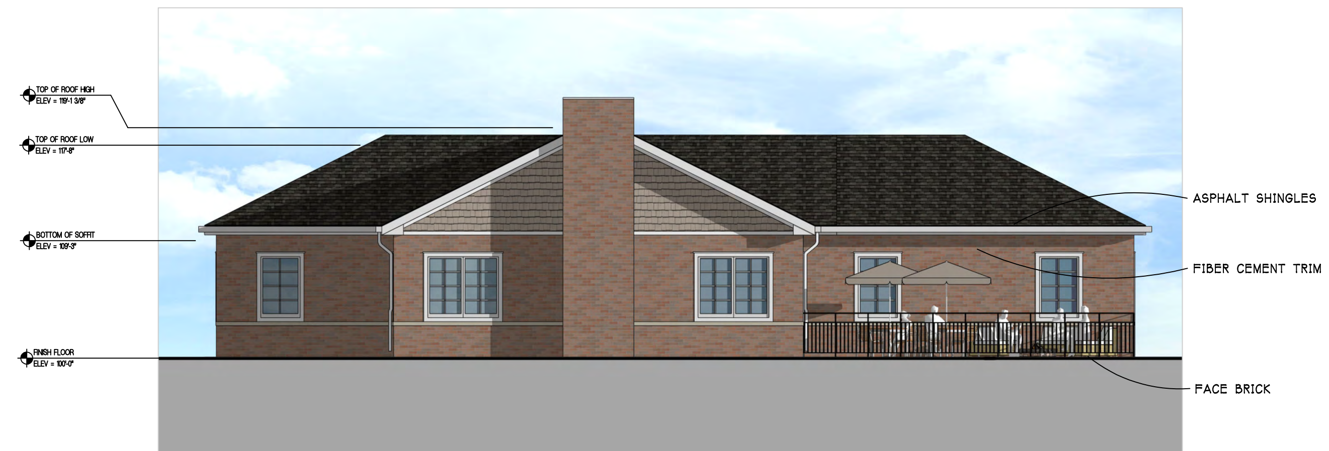
REAR ELEVATION: CLUBHOUSE SCALE - 1/8" = 1'-0" S48VAC201
