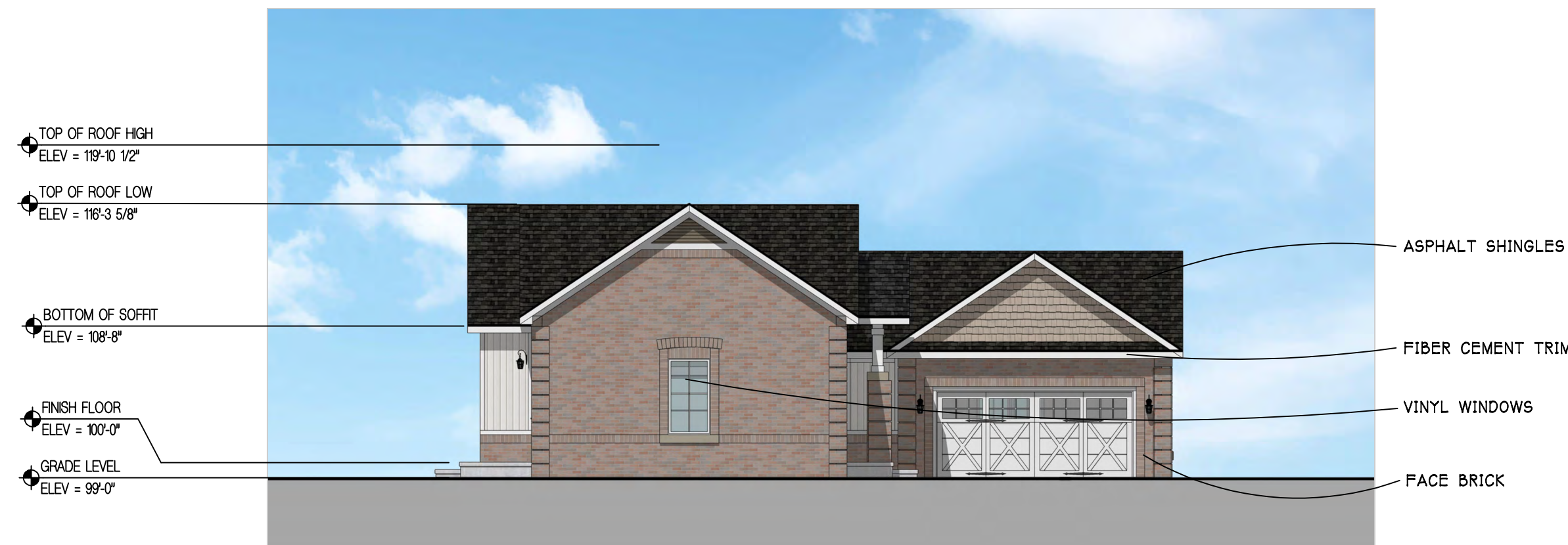
SIDE A ELEVATION UNIT B SCALE - 1/8" = 1'-0" SASHA.022
