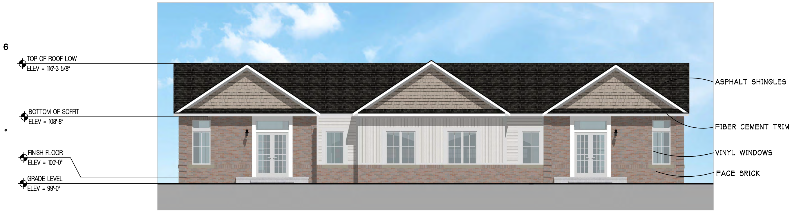
REAR ELEVATION: 2-UNIT A SCALE - 1/8" = 1'-0" SASHL021
