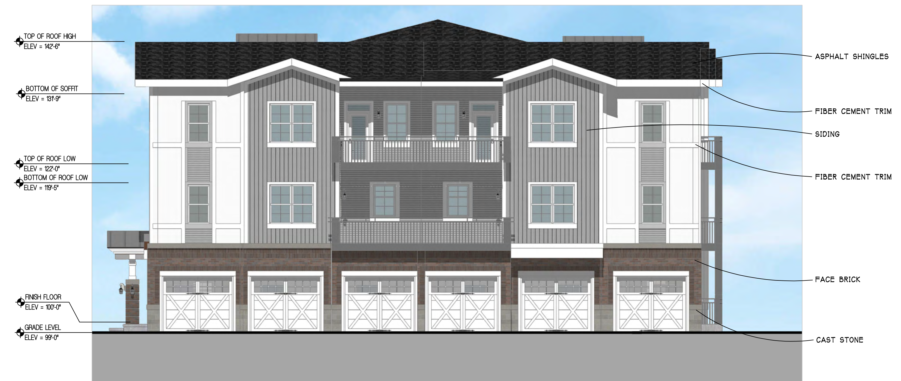
SIDE A ELEVATION: STACKED FLATS
