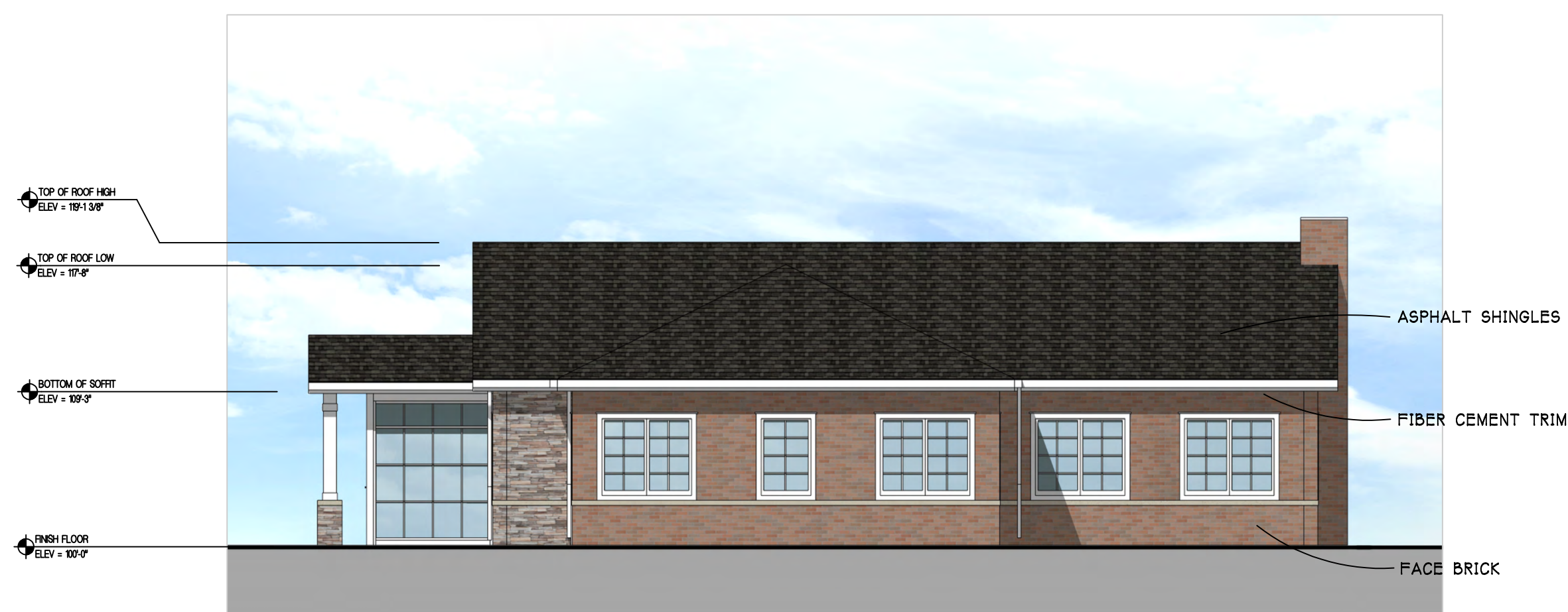
SIDE A ELEVATION: CLUBHOUSE SCALE - 1/8" = 1'-0" S48VAC201
