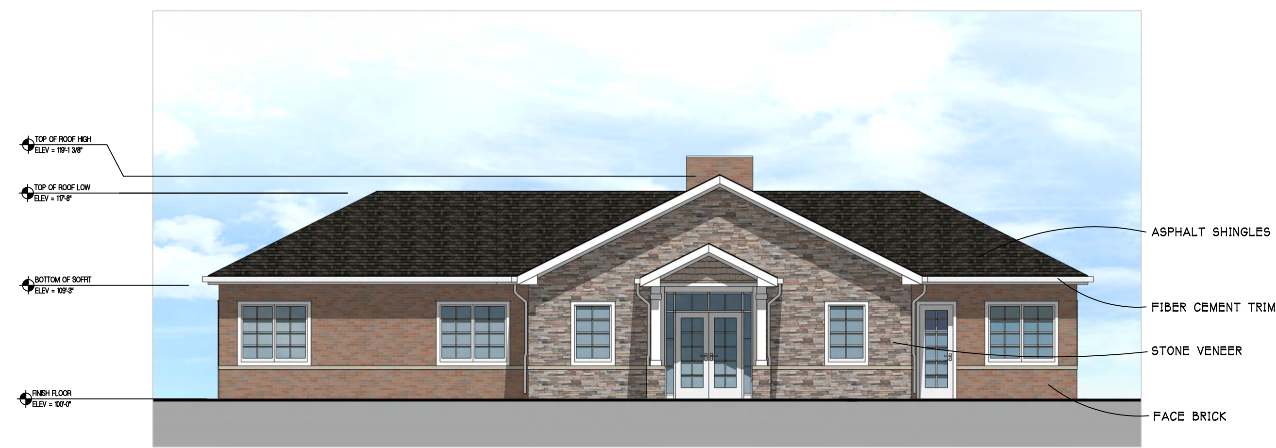
FRONT ELEVATION: CLUBHOUSE SCALE - 1/8" = 1'-0" S48VAC201
