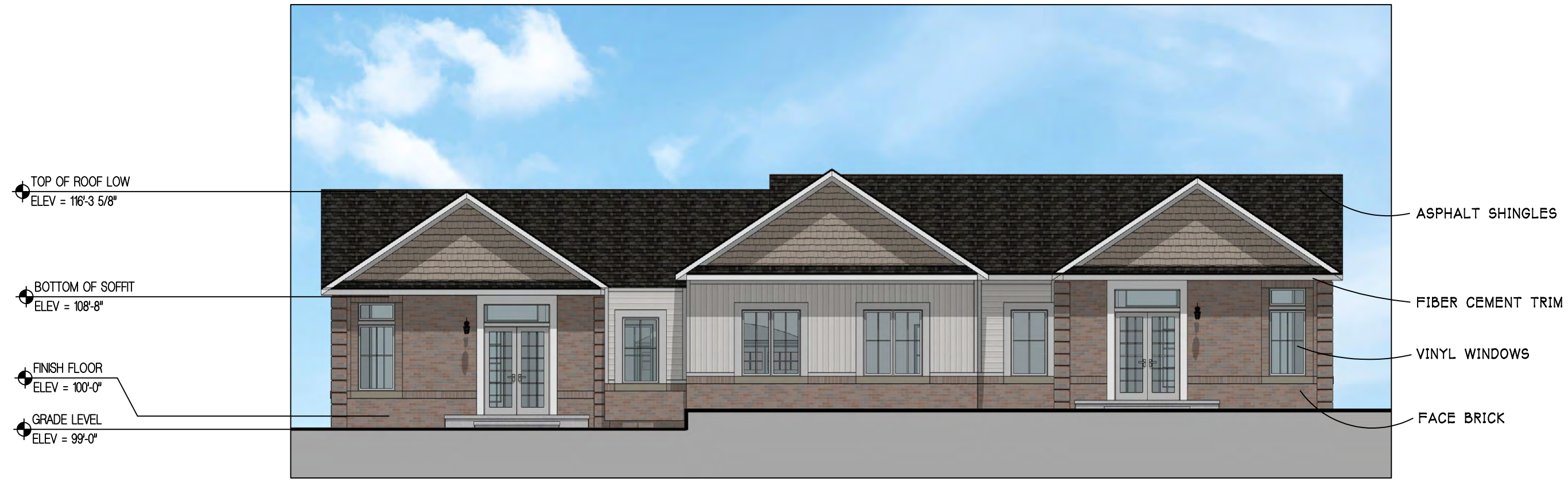
REAL ELEVATION: 2-UNIT B SCALE - 1/8" = 1'-0" SASHA.022
