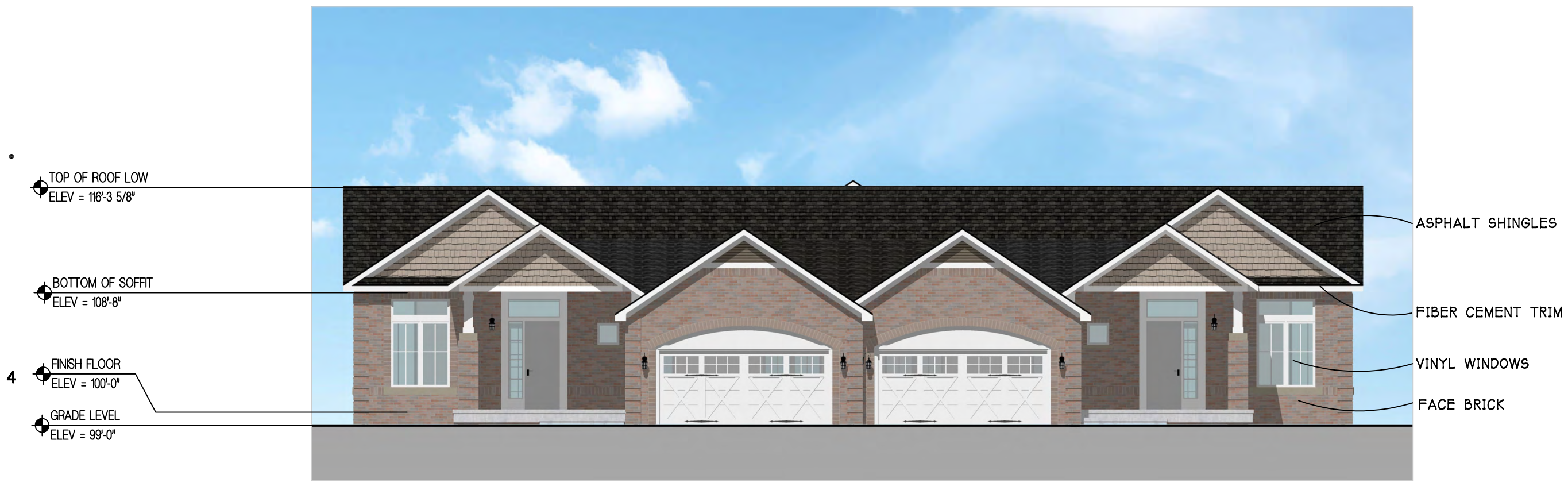
FRONT ELEVATION: 2-UNIT A SCALE - 1/8" = 1'-0" SASHL021
