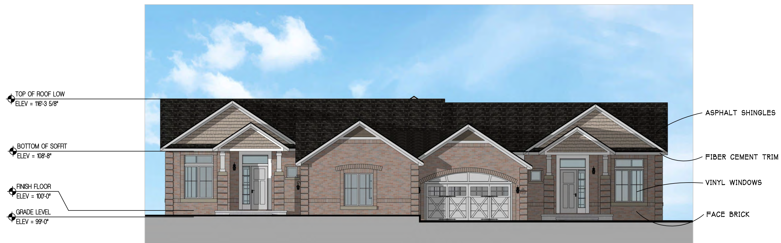
FRONT ELEVATION: 2-UNIT B SCALE - 1/8" = 1'-0" SASHA.022
