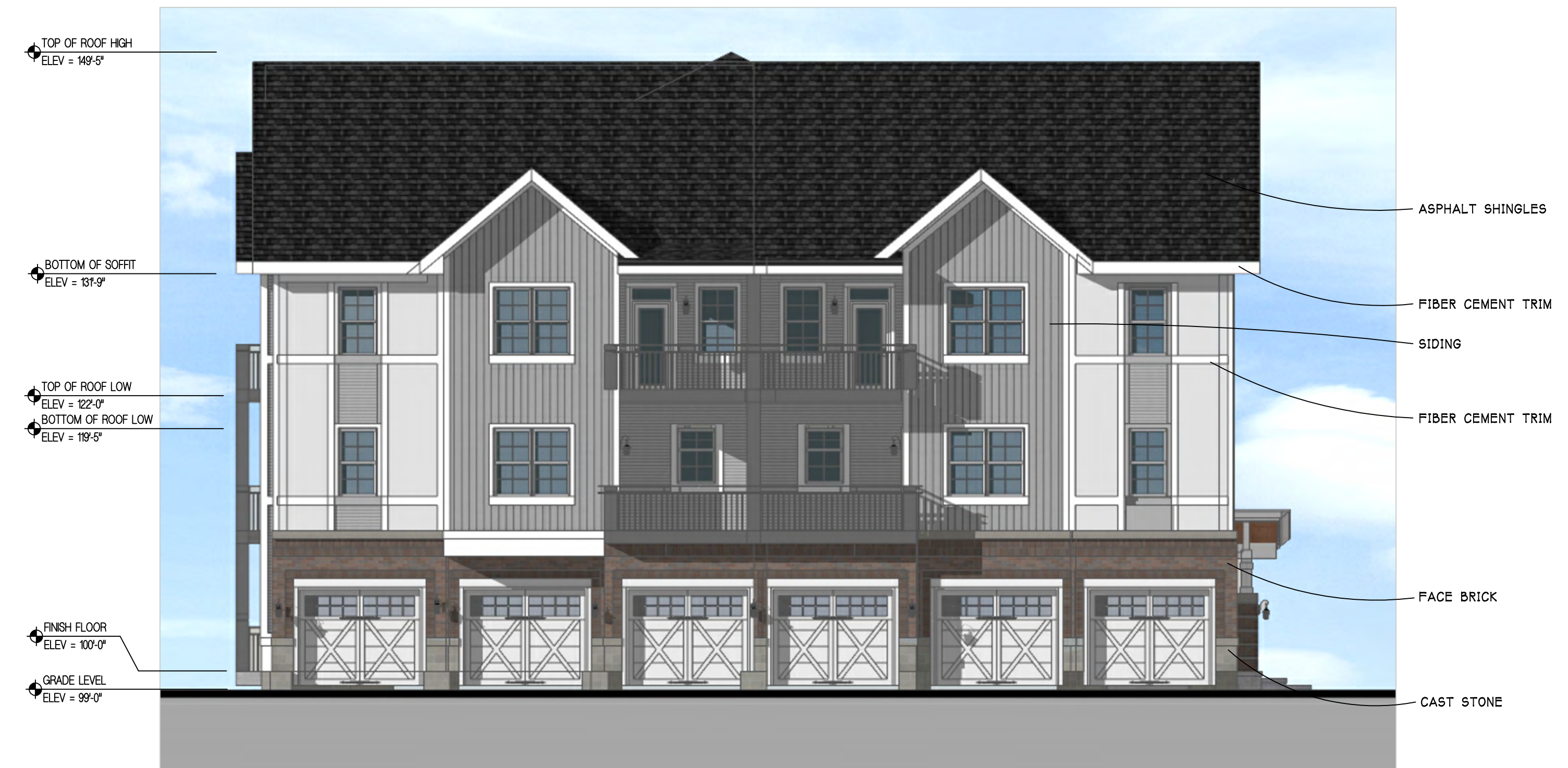
SIDE B ELEVATION: STACKED FLATS SCALE - 1/8" = 1'-0" S43W202
