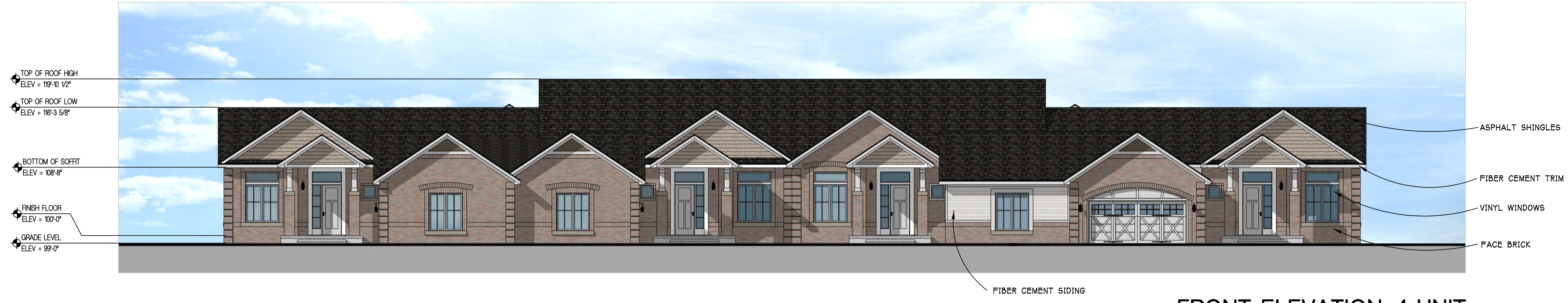
FRONT ELEVATION: 4-UNIT SCALE - 1/8" = 1'-0" SASHU202
