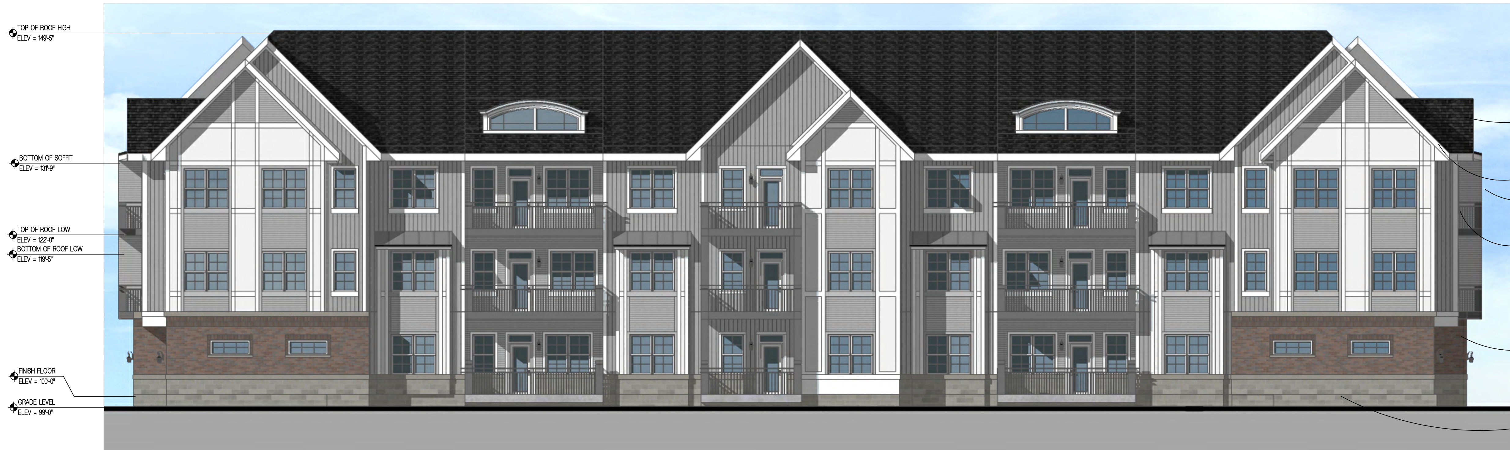
REAR ELEVATION: STACKED FLATS SCALE - 1/8" = 1'-0" 9/3/2021
