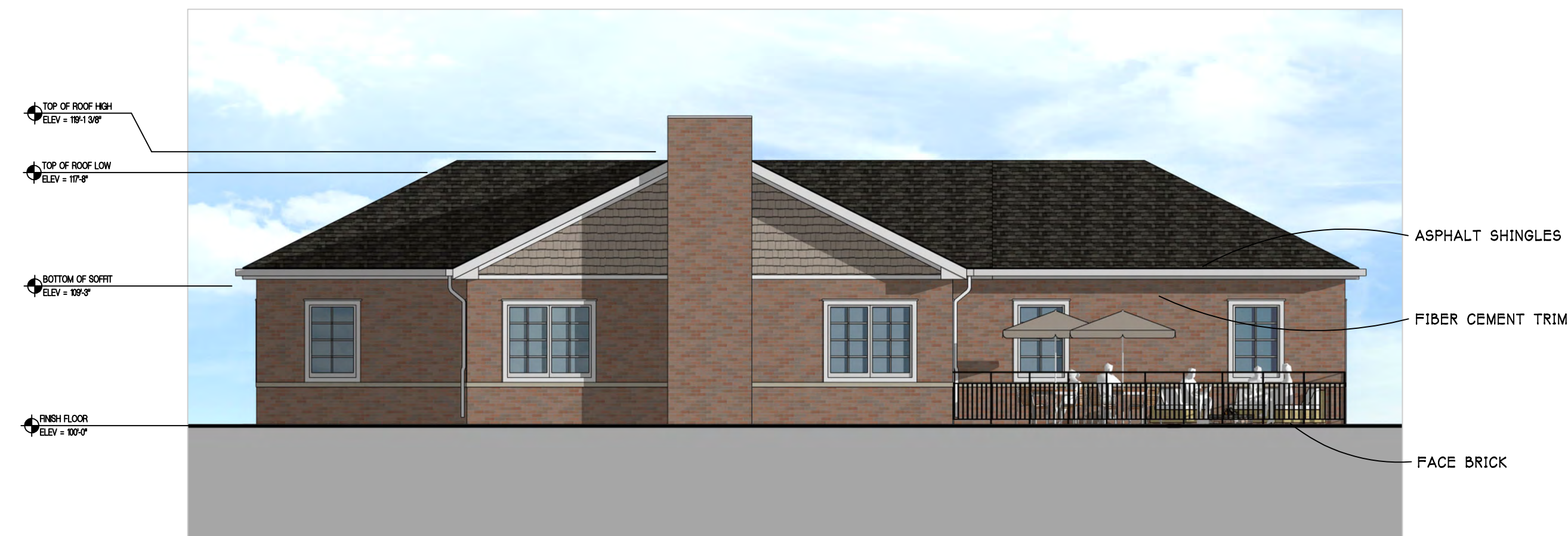
REAR ELEVATION: CLUBHOUSE SCALE - 1/8" = 1'-0" S48VAC201
