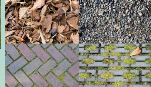
PERMEABLE PARKING LOT PAVING OPTIONS
