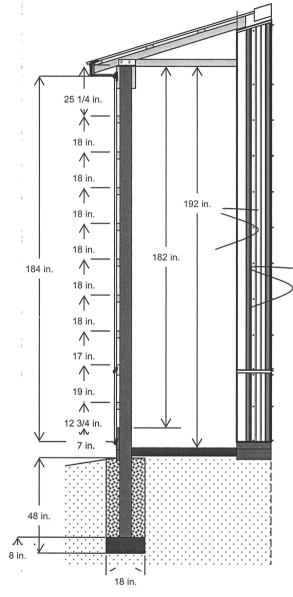
4/12 PITCH TRUSS SYSTEM WITH A STANDARD HEEL (HEEL HEIGHT: 0-3-15 OR 4 IN.) TRUSS SPACING: 24 IN. O.C. TRUSS LOADING INFORMATION: TCLL/TCDL/BCLL/BCDL 35-7-0-10 TOTAL TRUSS LOADING = 52 P.S.F. BRACE PER TRUSS MANUFACTURER'S RECOMMENDATIONS
